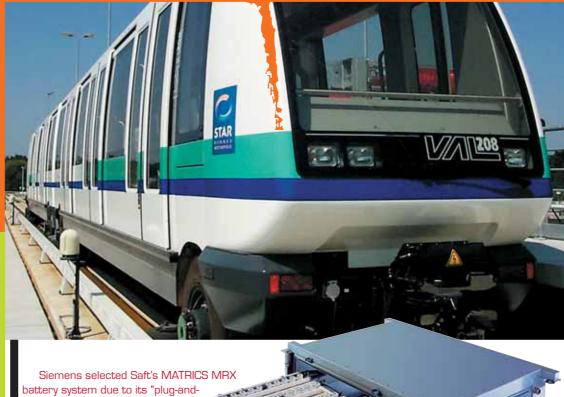
Siemens selected Saft's MATRICS battery system due to its "plug-and-play" capabilities, among other characteristics. The Saft battery provides backup power for the safety and auxiliary circuits of the trams, Siemens's new VAL 208.
