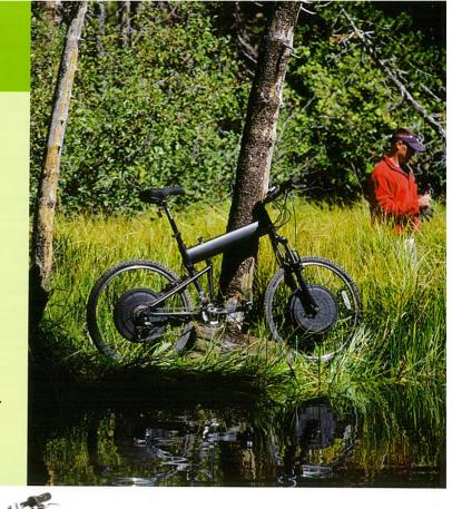
Originally aimed at security forces, the TidalForce M-750 (as WaveCrest's first electric bike is called) is a rugged, durable and foldable electric mountain bike. In the back hub is its patented WaveCrest Adaptive Motor system, and in the front hub are the Saft Ni-MH batteries composed of Saft's VH D cells. "We've created superior, reliable and unique bicycles powered by the newest wave in transportation technology," says Roy Barbee, WaveCrest's president and CEO.
