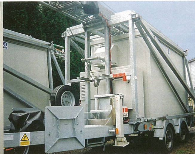
Above: a transportable GSM base station equipped with Ericsson radio transceivers and Saft Ni-Cd batteries. Left, a fixed base station on the Pacific Rim with Siemens infrastructure — and Saft Ni-Cds.
