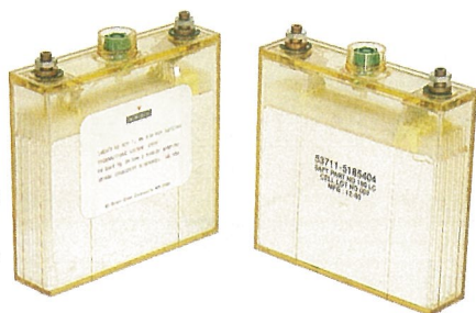
Silver oxide-zinc cells developed in the U.S. for underwater applications
