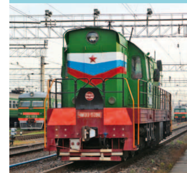
RZhD diesel loco type ChME3 equipped with Saft starting batteries
