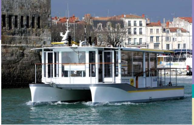
because the solar panels on the cabin roof provide up to 20% of the power needed.
